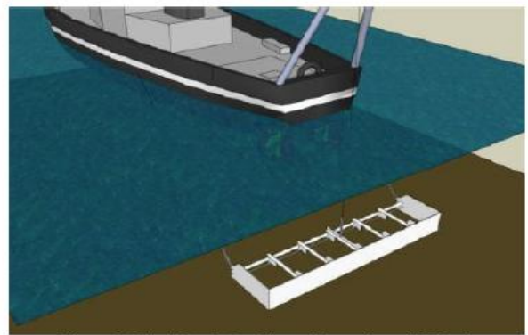
Figure 3. Principle of ploughing with a tugboat (H. Bots)
