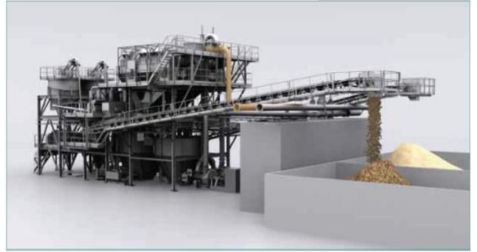
Figure 4. The AMORAS sand separation and washing plant
