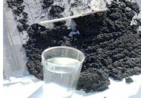
Figure 3. Flocculation Bench Scale Testing for the RDS
